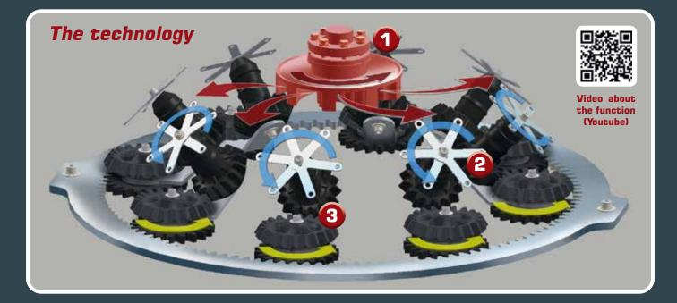
Processing takes place without compressed air according to the centrifugal wheel principle, in which the workpieces rotate on a satellite holder around a centrally arranged, **speed-controlled centrifugal wheel** ①.
