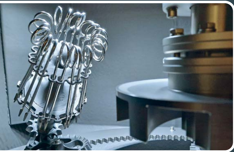
Workpieces in a BMF TWISTER blasting system on a 3D-printed workpiece carrier
