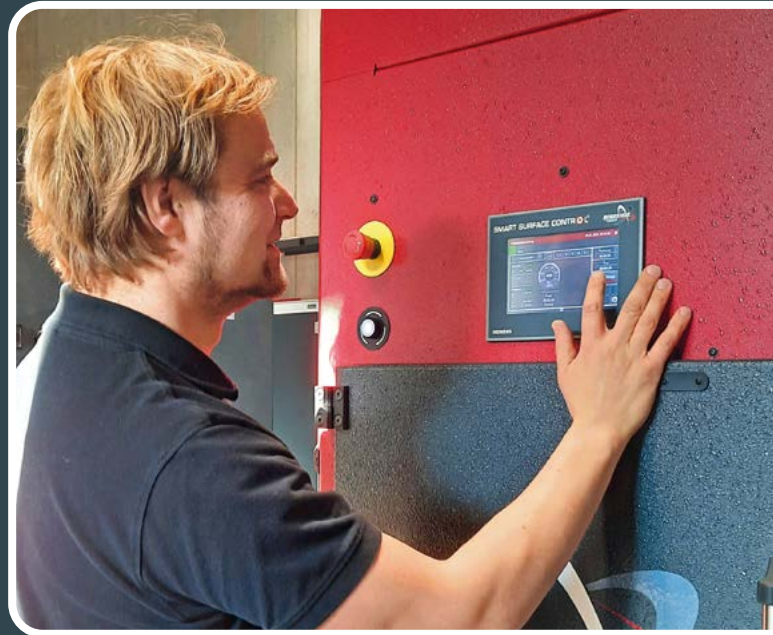
The desired blasting parameters are entered quickly and easily on a touch panel
